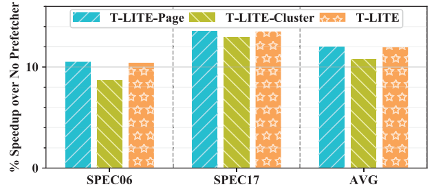
Fig. 15: With behavioral clustering , a fine-tuning pass recalibrates T-LITE to take clusters as inputs instead of pages.
